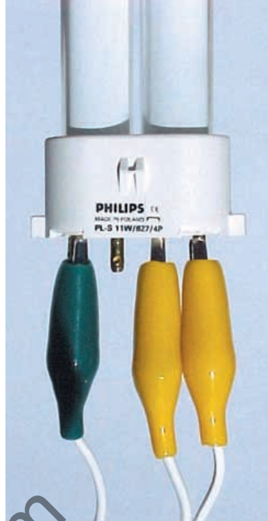
Test clips on an 11W c.f.l. assembly.
