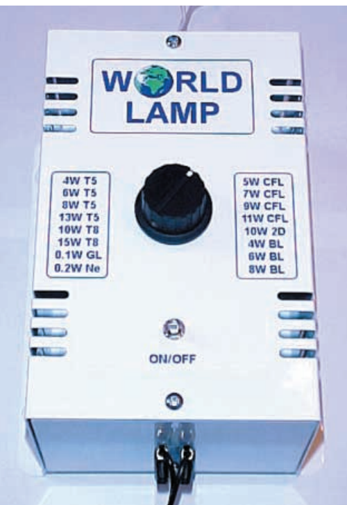
Completed World Lamp in a robust well-ventilated metal case.
