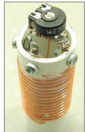
(Right) Completed tuning coil showing preset soldered to tags bolted on one end of former.
